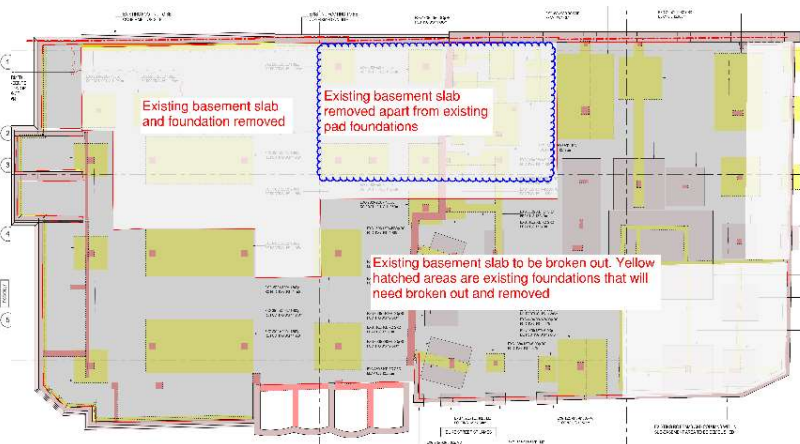
Progress up to date and direction of break out works
