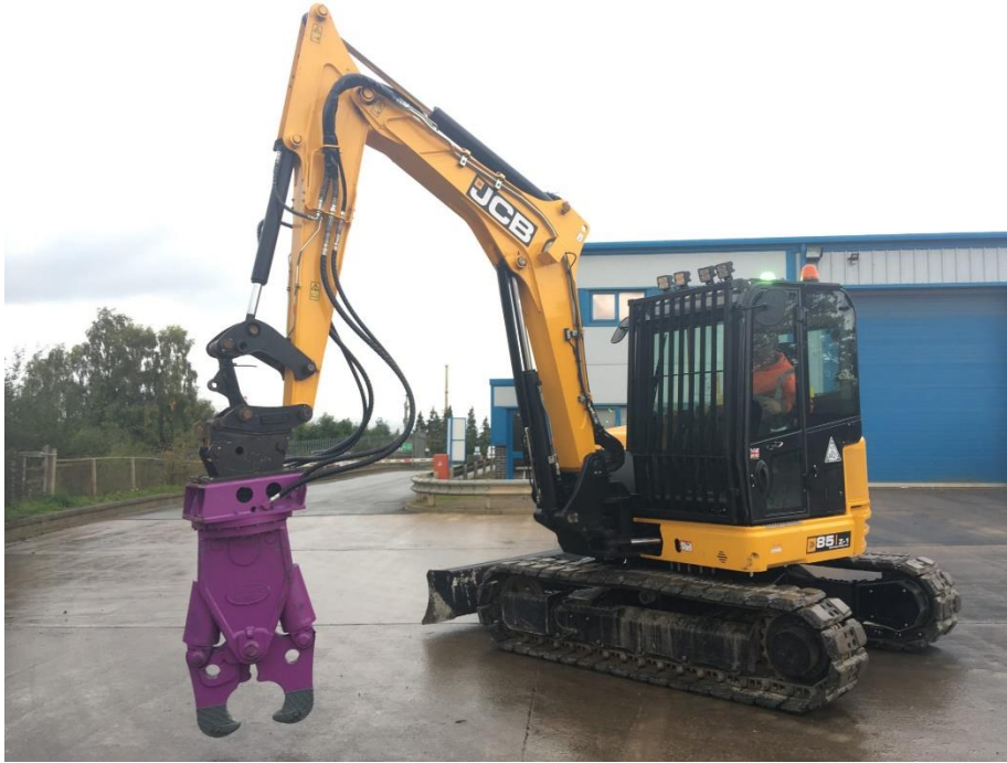
Typical excavator equipped with a concrete cracker attachment that will be used for demolition works
